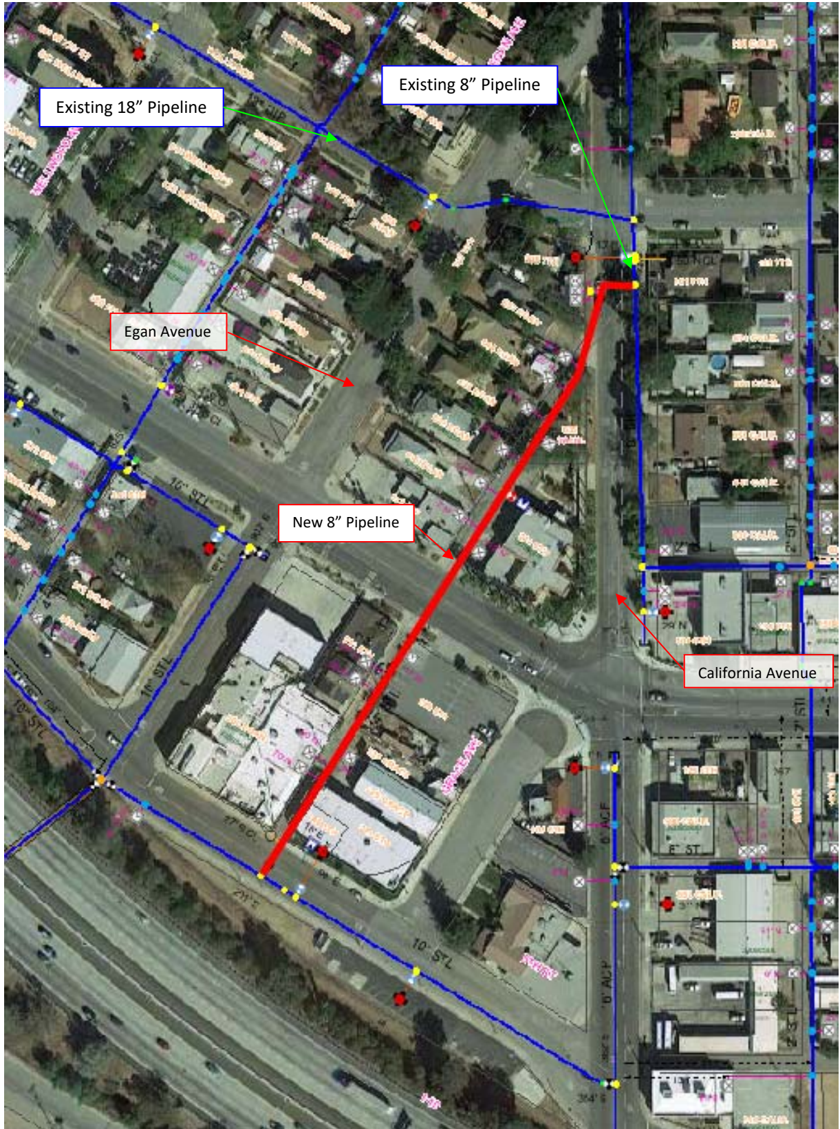
Figure 6: Replacement Pipeline 3 Site Map
